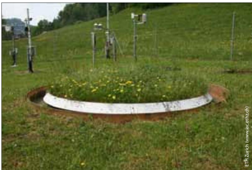
A lysimeter used to test evaporation with realistic environmental conditions.
