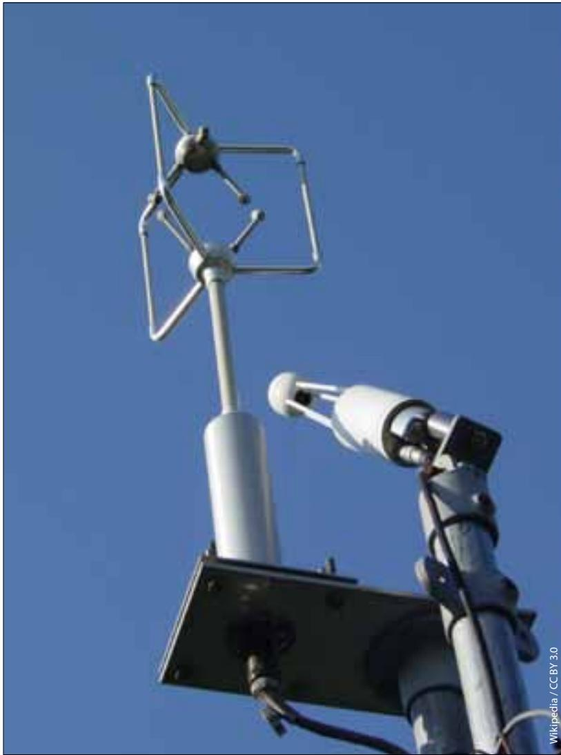
Eddy covariance system consisting of an ultrasonic anemometer and infrared gas analyser (IRGA).
