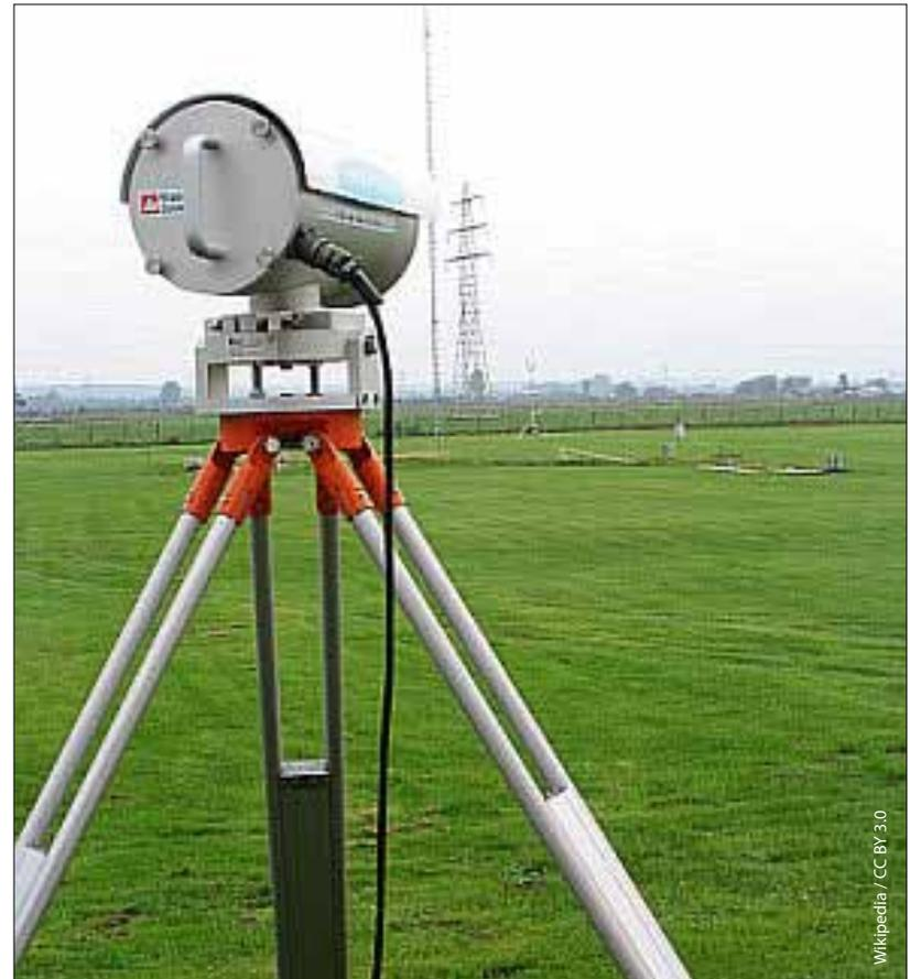
A Large Aperture Scintillometer (transmitter) for measurement of the sensible heat flux over long distances.
